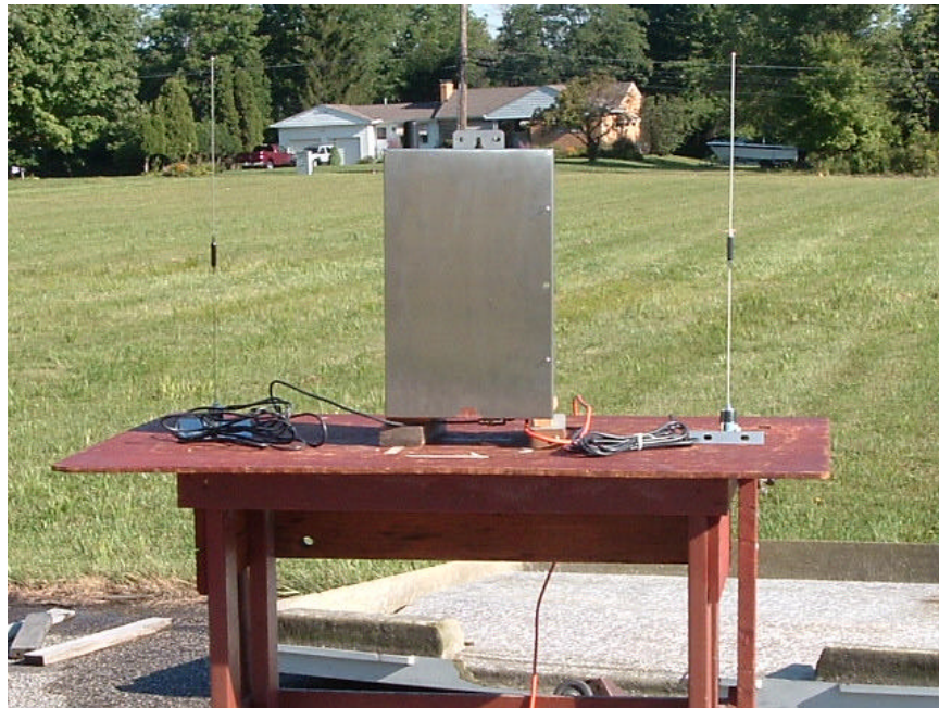
Radiated Emissions Test Set-up
