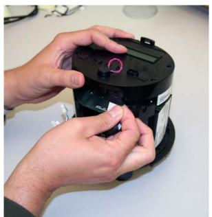
**Step 4** – Connect additional wiring to the faceplate as required for the specific meter configuration.
