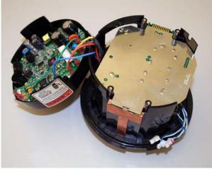
**Step 2** – Close the housing as shown here, aligning the faceplate with the mounting posts on the body of the housing.
