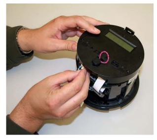
**Step 5** – Attach the faceplate to the body of the housing by inserting and tightening the required screws.
