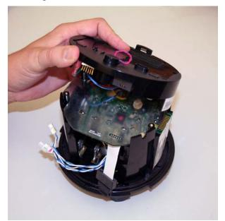
**Step 3** – Connect the MTU ribbon cable to the connector on the S4 Meter faceplate as shown below.
