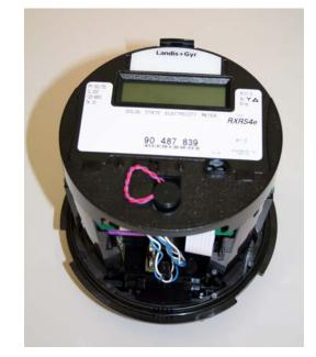
**Step 7** – Install the meter cover to complete the meter assembly.
