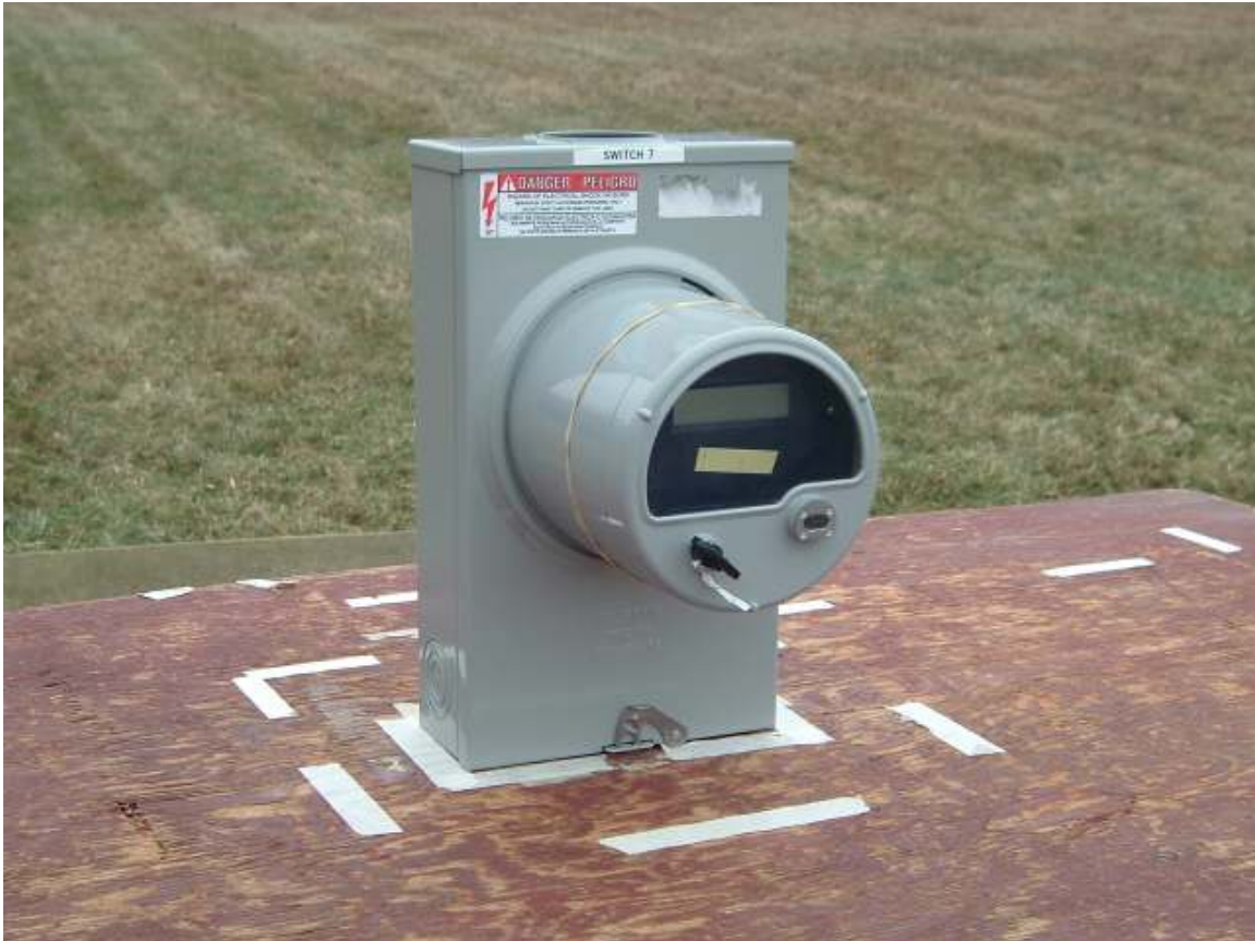
PICTORIAL 1 HEXAGRAM MODEL 9845 MTU OUTPUT POWER AND SPURIOUS EMISSIONS TYPICAL TEST SETUP
