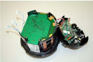
**Step 2** – Close the housing as shown here, aligning the faceplate with the mounting posts on the body of the housing.
