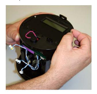
**Step 4** – Connect the MTU ribbon cable to the connector on the S4 Meter faceplate as shown below.
