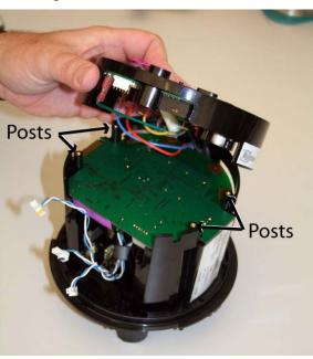
**Step 3** – Attach the faceplate to the body of the housing by inserting and tightening the required screws.
