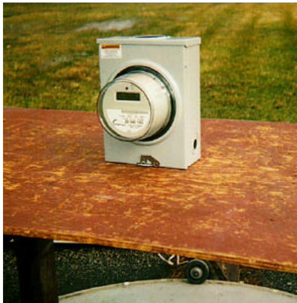
PICTORIAL 1 HEXAGRAM 8877PM ELECTRIC METER TRANSMITTING UNIT OUTPUT POWER AND SPURIOUS EMISSIONS TEST SETUP
