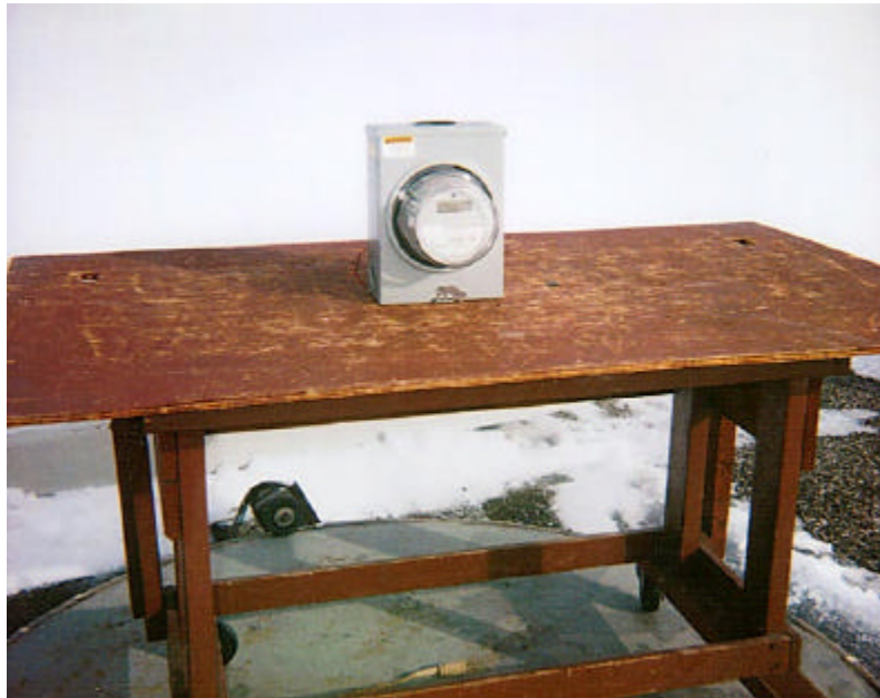
PICTORIAL 1 HEXAGRAM 8877P ELECTRIC METER TRANSMITTING UNIT OUTPUT POWER AND SPURIOUS EMISSIONS TEST SETUP
