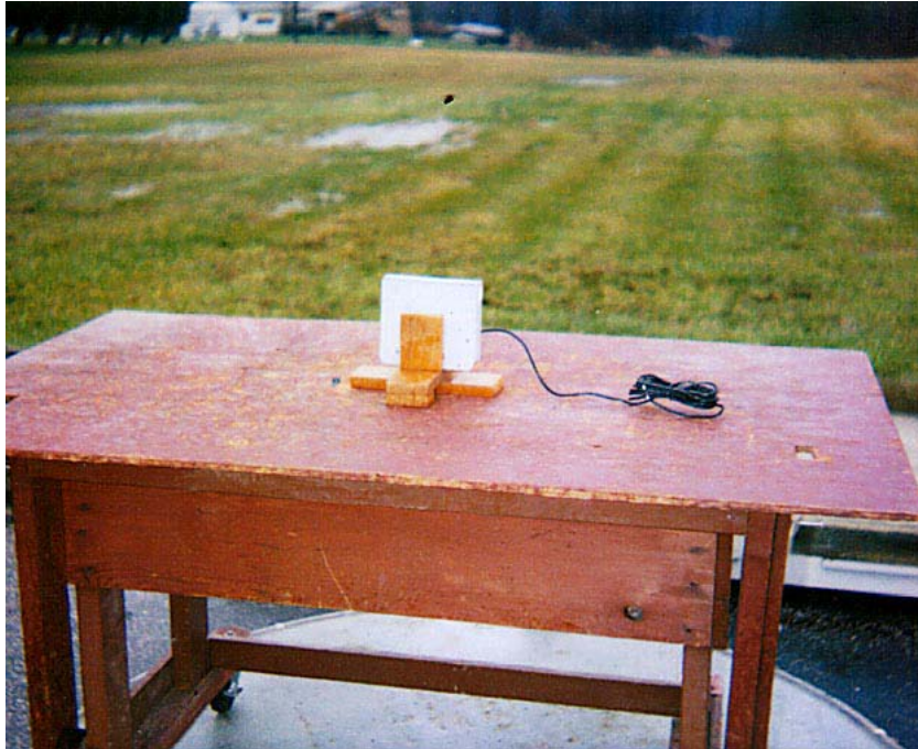
PICTORIAL 1a HEXAGRAM METER TRANSMITTING UNIT MODEL 6327PW, with external wiring OUTPUT POWER AND SPURIOUS EMISSIONS TEST SETUP
