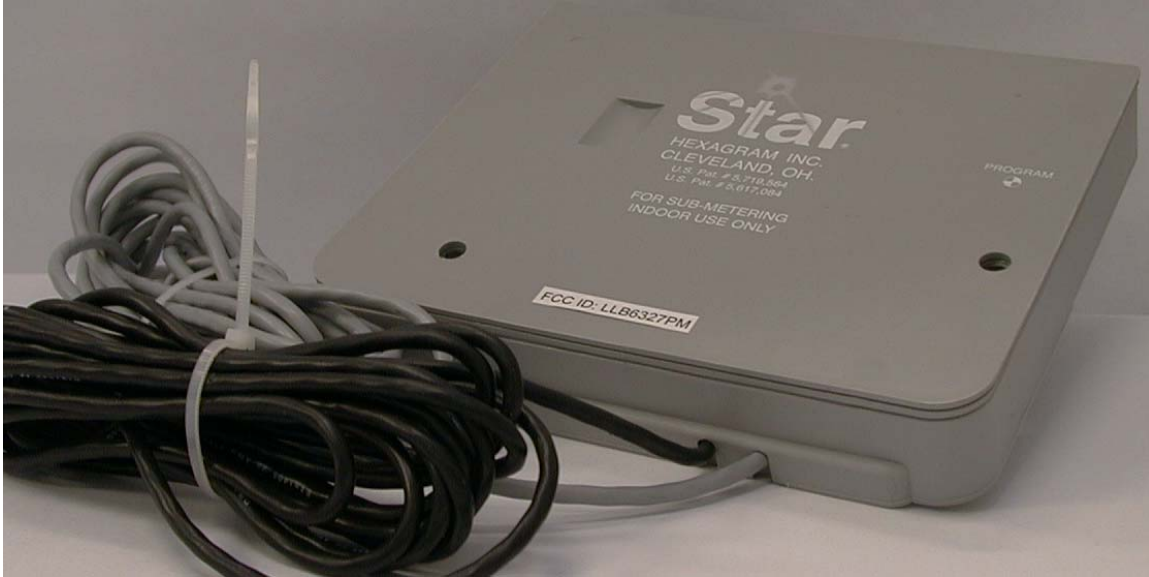
External Photos LLB6327PM MTUs with Two and One external wires
