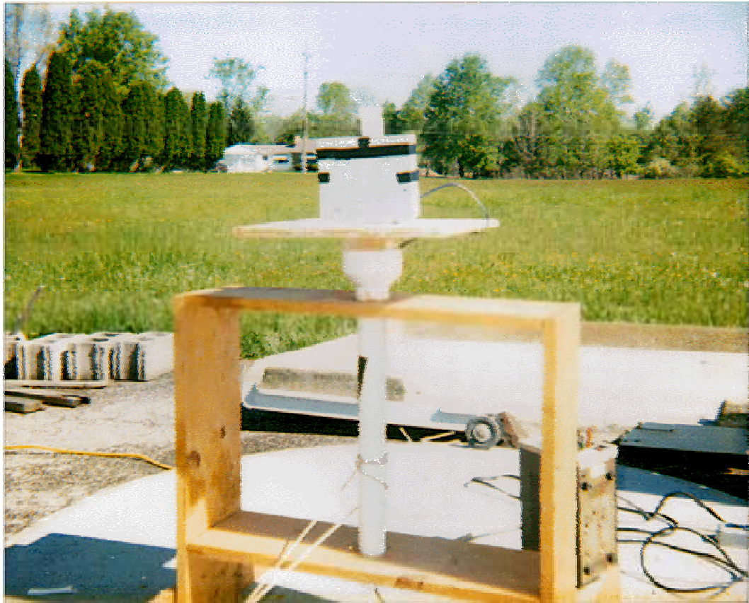
Photo 1 Hexagram, Inc. "Flatpac" Transmitter Emissions Test Set-Up
