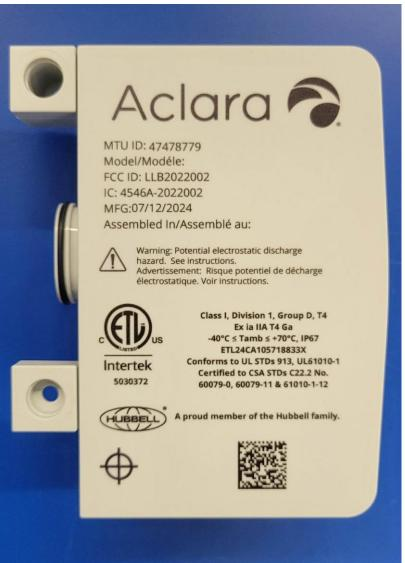
See below for the actual label. The model is listed in the next drawing. The label is printed directly onto the plastic housing. The dimensions of the plastic housing are 3.76 inches by 4.72 inches.
