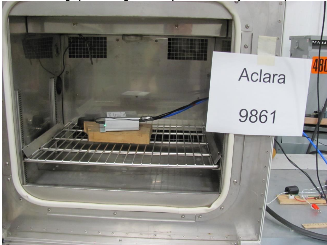
Photograph of Voltage and Temperature Stability Test Setup
