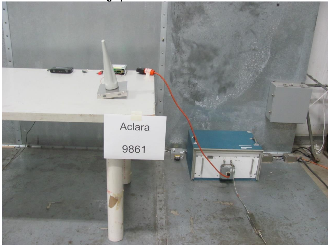
Photograph of AC conducted Emissions
