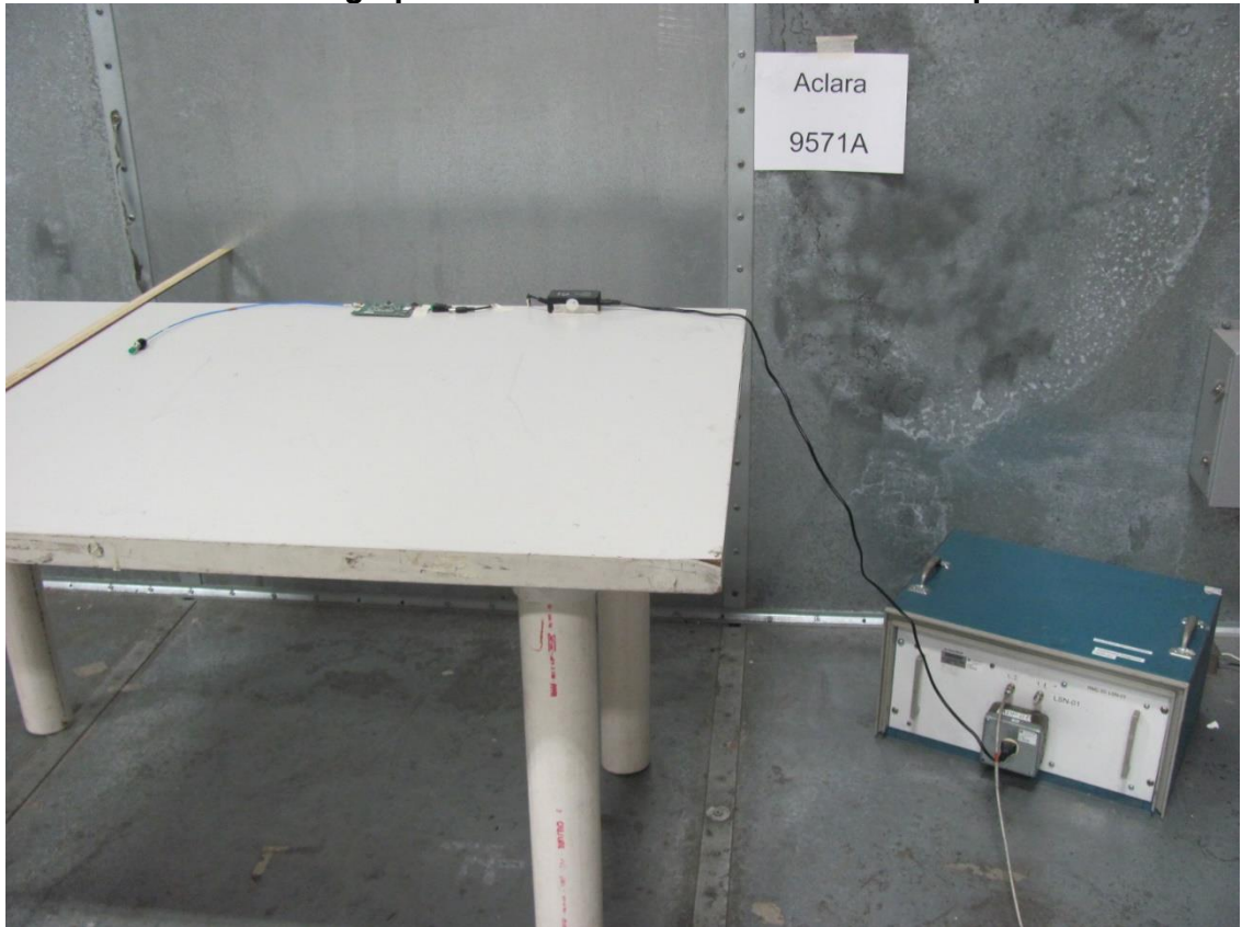
Photograph of Conducted Emissions Test Setup
