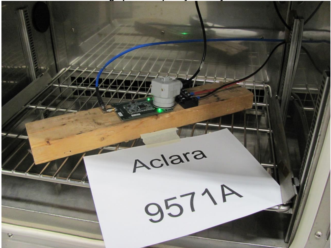
Photograph of Frequency Stability tests
