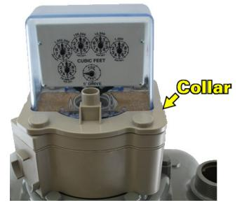
**4.** Secure the index and collar to the MTU using the #10-32 X 1" screws. Tighten both screws to 2-3 inch-pounds.
