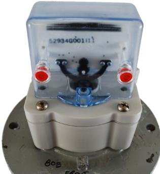
2. Align the index drive with the MTU gear.
