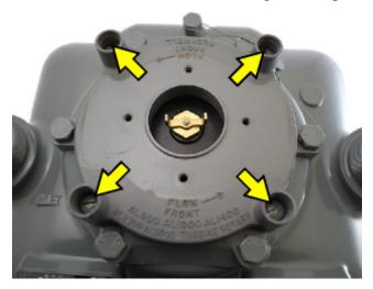
**NOTE:** If more than two screws are broken, or if two screws are broken and they are not on opposite diagonal sides, the MTU <u>should not</u> be installed.
