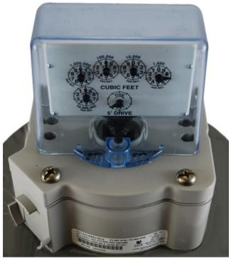
NOTE: On some older meters, like the 60B and 80B, the index and MTU must be installed so that the dials and puck retention collar face the rear of the meter, as shown.
