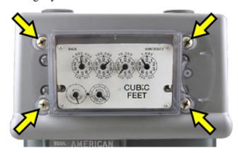
**CAUTION!** Do not over tighten screws. Excessive torque may damage the MTU enclosure.
