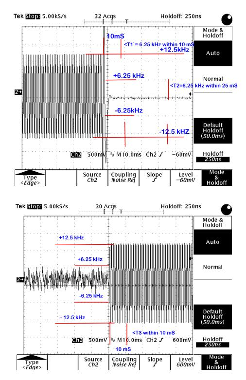
**Test Requirements:** Frequency deviation during  $t_1$  (10 ms duration after  $t_{on}$ ) may be greater than ±12.5 kHz because the output power is less than 6 Watts. Frequency deviation during  $t_2$  (25 ms duration after  $t_1$ ) must be less than ±6.25 kHz. 3. Frequency deviation after  $t_2$  must be less than ±2.5 ppm, or ±1150 Hz at 460 MHz. Frequency deviation during  $t_3$  (10 ms duration after transmitter is turned off) may exceed ±12.5 kHz because output power is less than 6 Watts.
