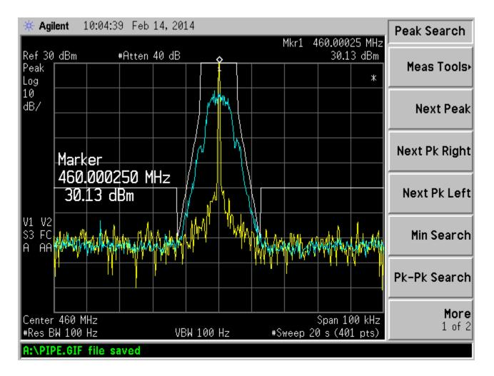
The above plot demonstrates that the EUT meets the 90.210 Emission Mask D requirements:
