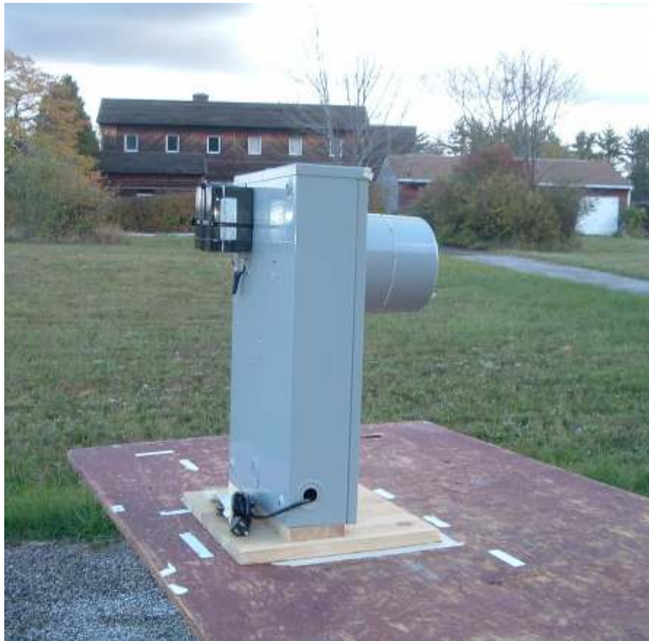
PICTORIAL 1 HEXAGRAM MODEL 14973 MTU OUTPUT POWER AND SPURIOUS EMISSIONS TYPICAL TEST SETUP
