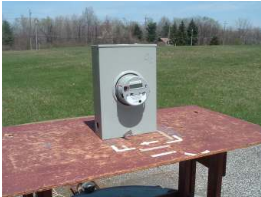
PICTORIAL 1 HEXAGRAM MODEL 14280 MTU OUTPUT POWER AND SPURIOUS EMISSIONS TYPICAL TEST SETUP
