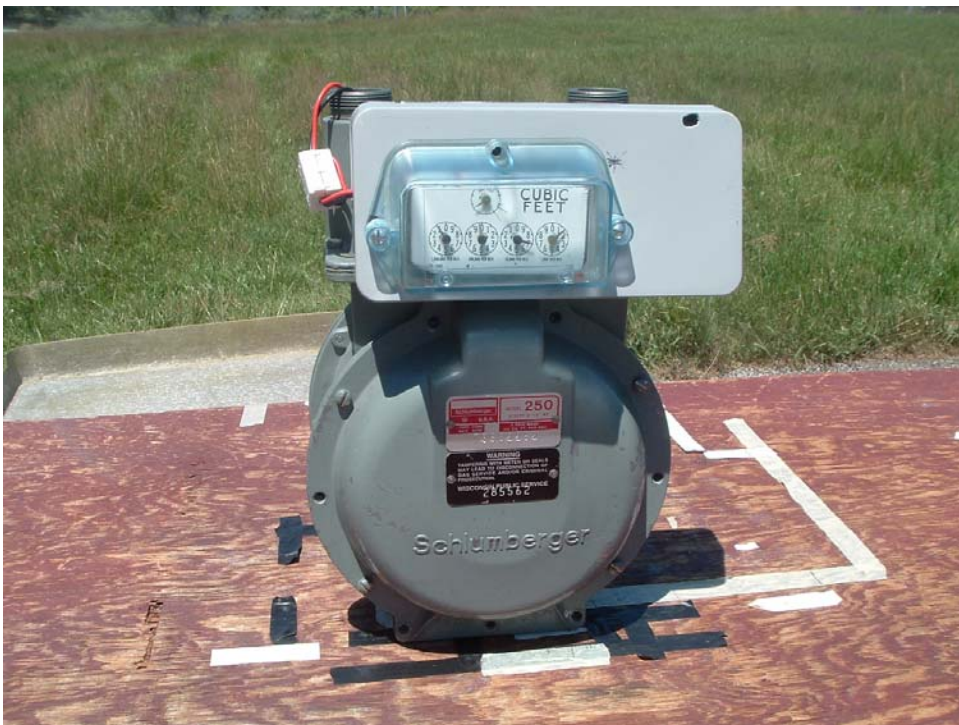
PICTORIAL 1 HEXAGRAM MODEL 11583-2 MTU OUTPUT POWER AND SPURIOUS EMISSIONS TYPICAL TEST SETUP
