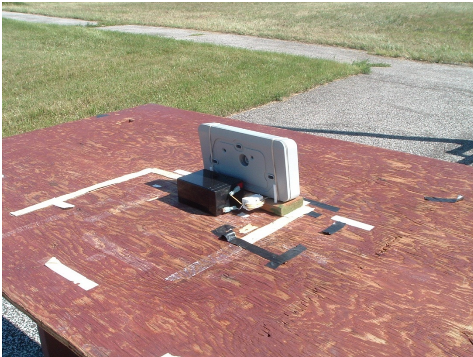
PICTORIAL 2 HEXAGRAM MODEL 2011-009X MTU OUTPUT POWER AND SPURIOUS EMISSIONS TYPICAL TEST SETUP
