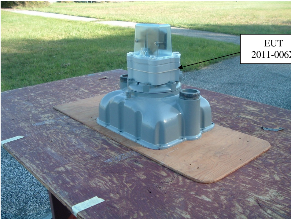
PICTORIAL 2 HEXAGRAM MODEL 2011-006X MTU OUTPUT POWER AND SPURIOUS EMISSIONS TYPICAL TEST SETUP
