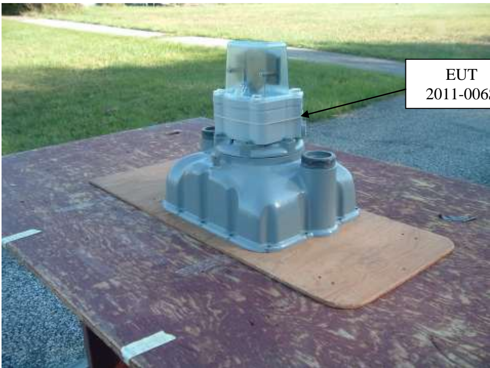
PICTORIAL 2 HEXAGRAM MODEL 2011-006S MTU OUTPUT POWER AND SPURIOUS EMISSIONS TYPICAL TEST SETUP
