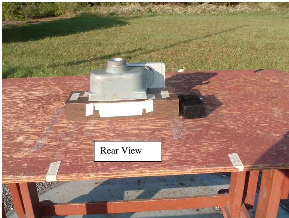
PICTORIAL 2 HEXAGRAM MODEL 2010-004S MTU OUTPUT POWER AND SPURIOUS EMISSIONS TYPICAL TEST SETUP
