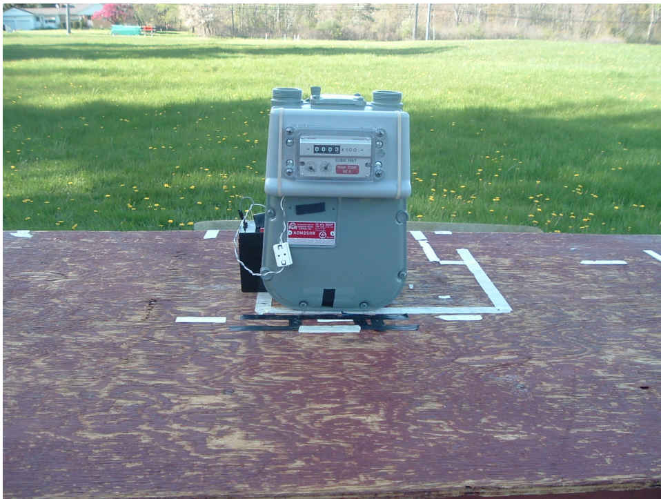
PICTORIAL 1 HEXAGRAM MODEL 2010-001, Rev G MTU OUTPUT POWER AND SPURIOUS EMISSIONS TYPICAL TEST SETUP
