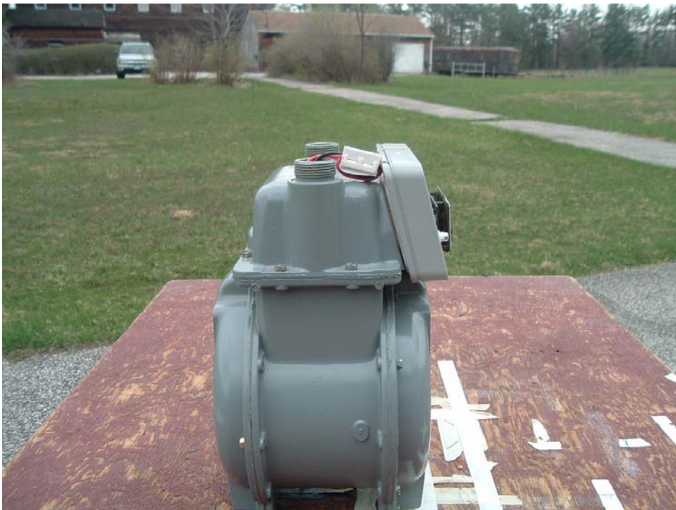
PICTORIAL 1 HEXAGRAM MODEL 2009-015 MTU OUTPUT POWER AND SPURIOUS EMISSIONS TYPICAL TEST SETUP
