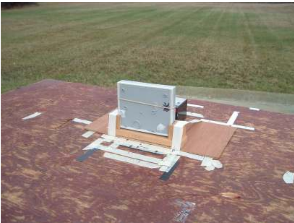
PICTORIAL 1 HEXAGRAM MODEL 2009-014 MTU OUTPUT POWER AND SPURIOUS EMISSIONS TYPICAL TEST SETUP
