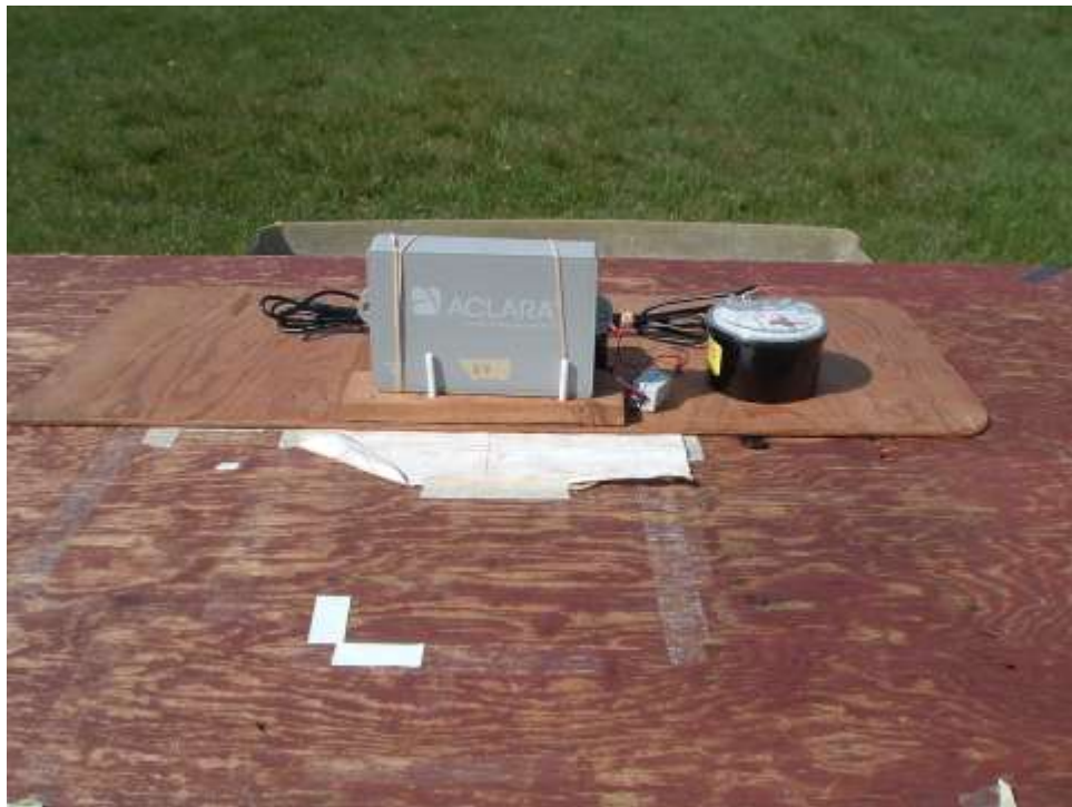
PICTORIAL 1 HEXAGRAM MODEL 2009-010B4, MTU OUTPUT POWER AND SPURIOUS EMISSIONS TYPICAL TEST SETUP
