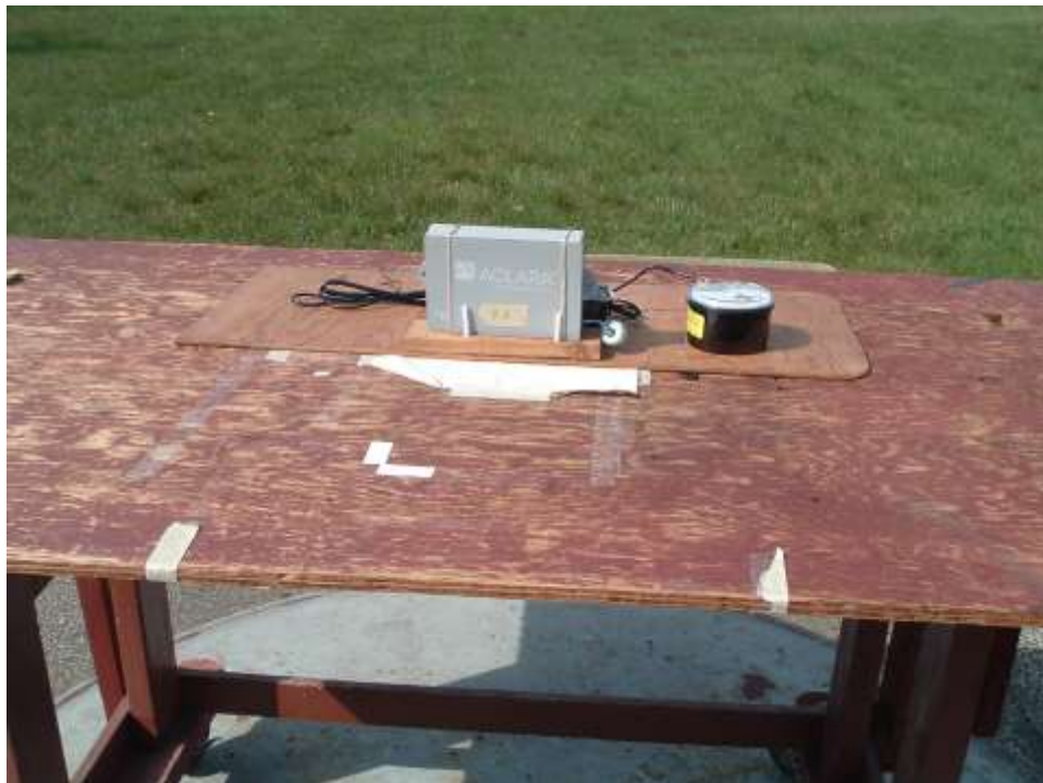
PICTORIAL 1 HEXAGRAM MODEL 2009-010B2, MTU OUTPUT POWER AND SPURIOUS EMISSIONS TYPICAL TEST SETUP
