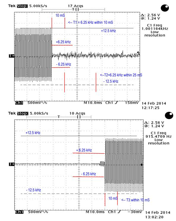
**Test Requirements:** Frequency deviation during  $t_1$  (10 ms duration after  $t_{on}$ ) may be greater than ±12.5 kHz because the output power is less than 6 Watts. Frequency deviation during  $t_2$  (25 ms duration after  $t_1$ ) must be less than ±6.25 kHz. 3. Frequency deviation after  $t_2$  must be less than ±2.5 ppm, or ±1150 Hz at 460 MHz. Frequency deviation during  $t_3$  (10 ms duration after transmitter is turned off) may exceed ±12.5 kHz because output power is less than 6 Watts.
