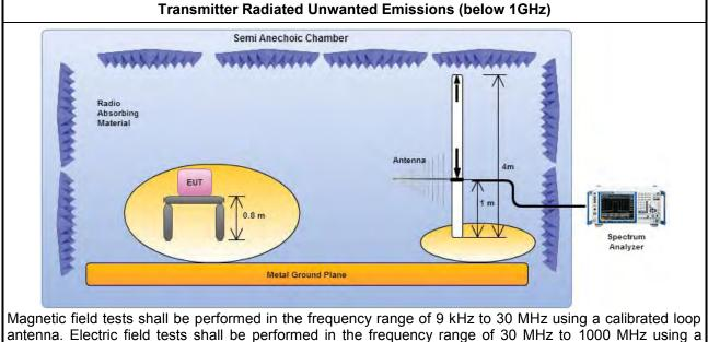
antenna. Electric field tests shall be perforn calibrated bi-log antenna.
