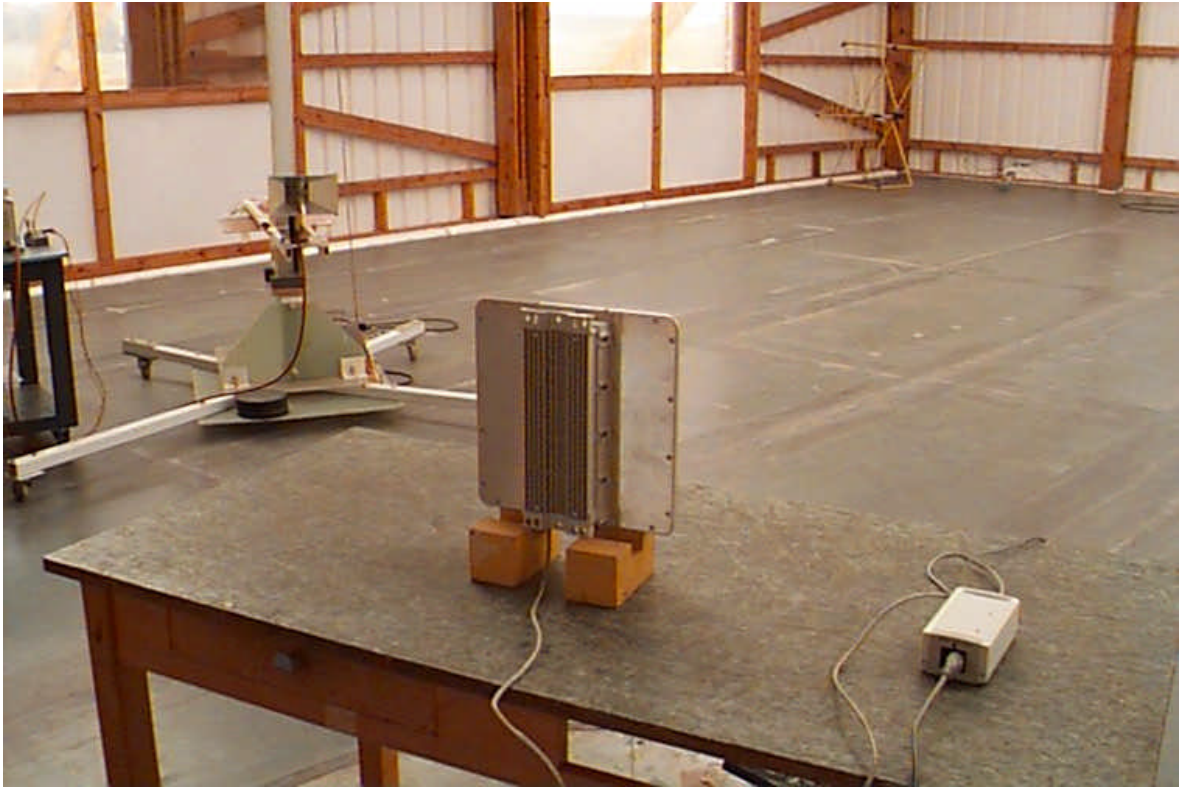
Photograph 4.5.1 Radiated spurious emissions measurement setup at the open field test site
