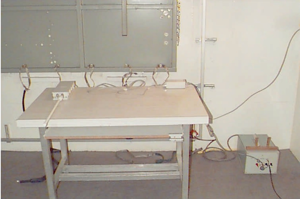
Photograph 4.8.1 Conducted emission measurements test setup
