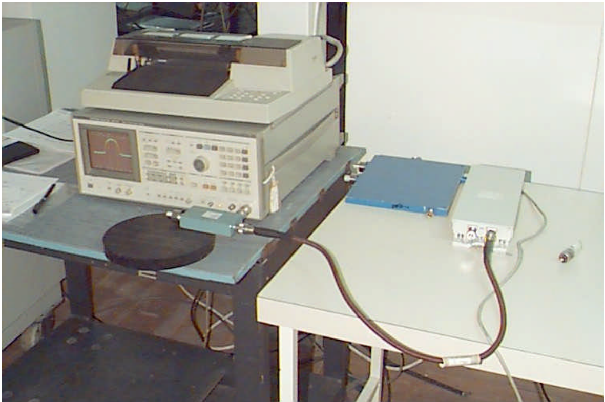
Photograph 4.1.1 Setup for minimum bandwidth measurements
