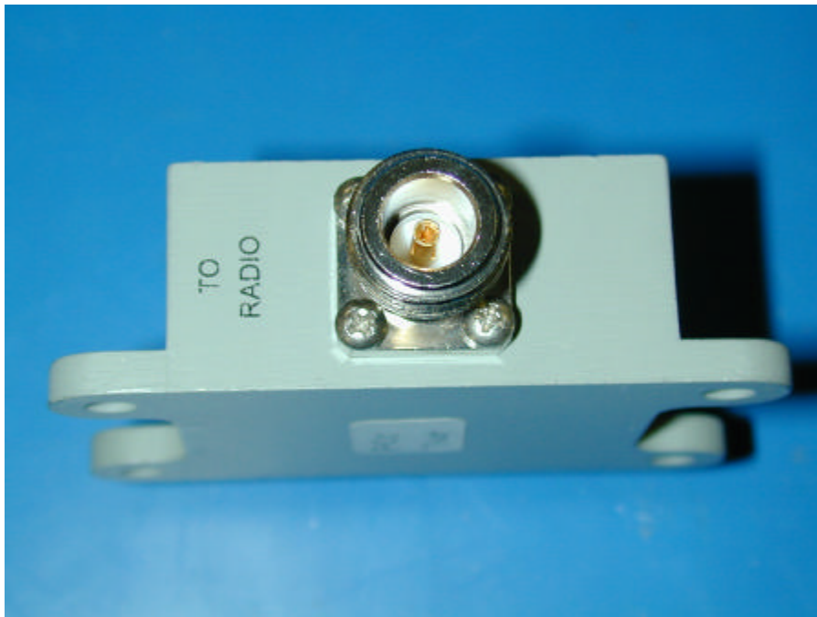
DC POWER INJECTOR REAR VIEW
