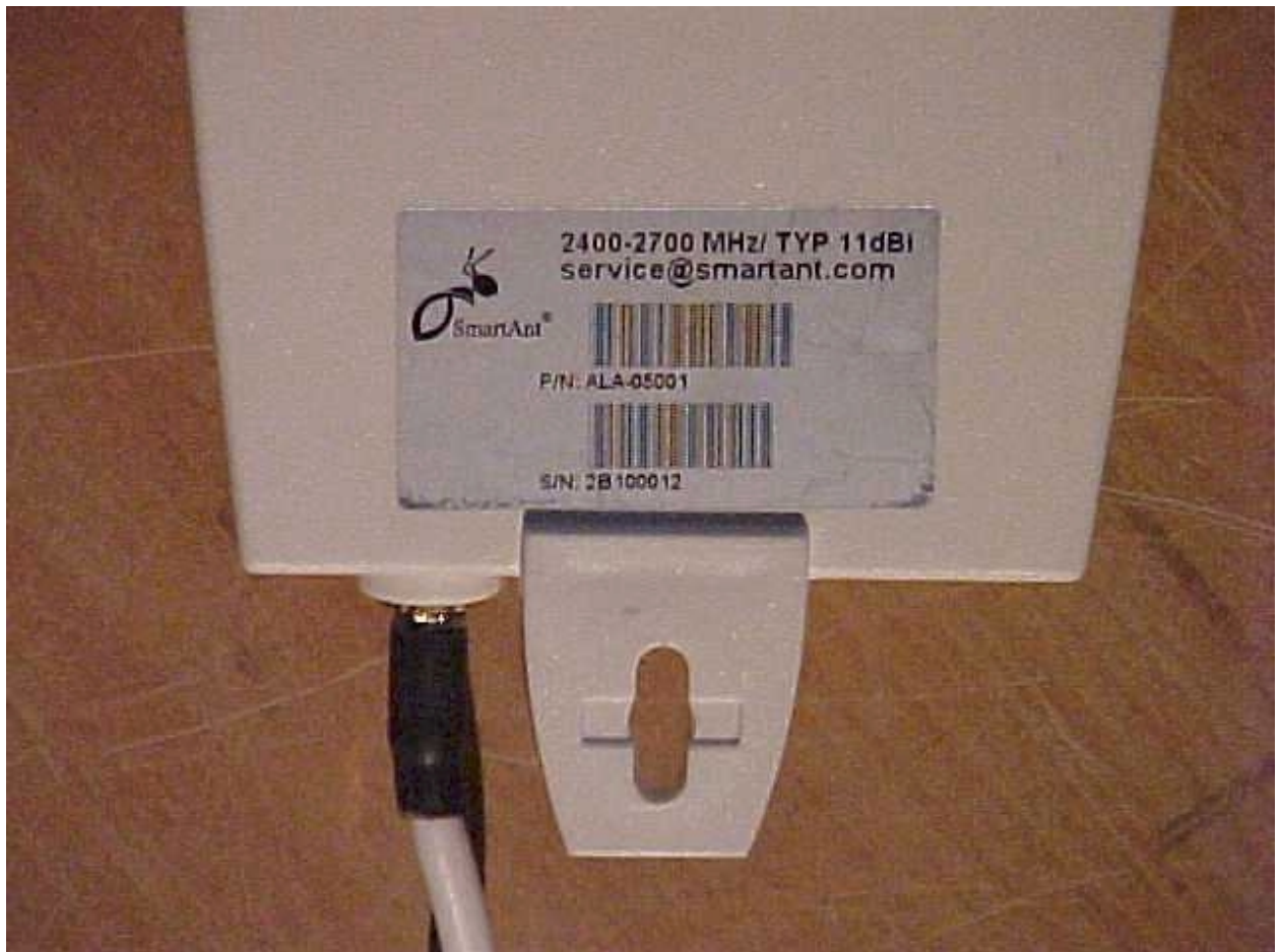
Photo #5 Antenna 2400-2700 MHz/TYP 11dBi
