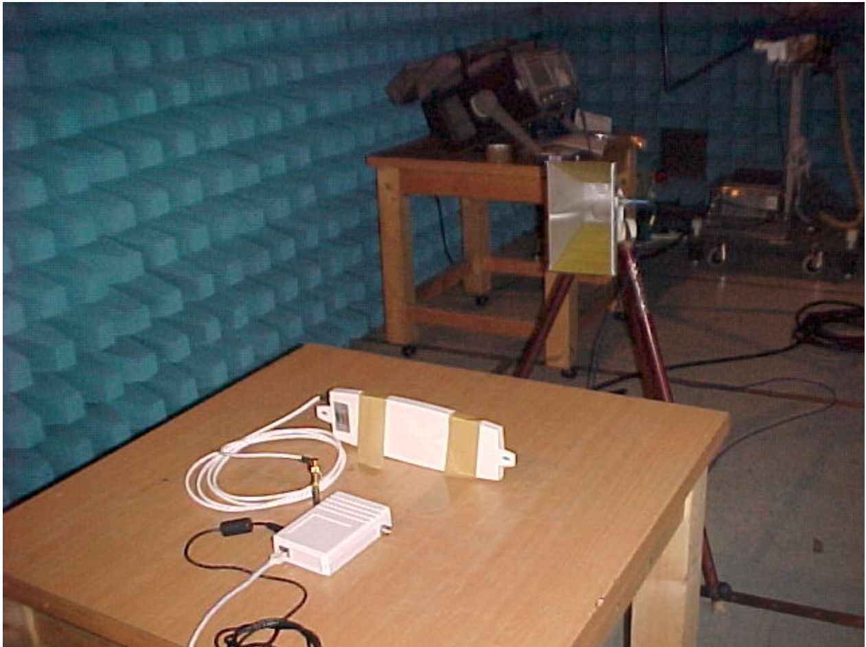
Photo #4 One Box 2.4 GHz Radio test setup
