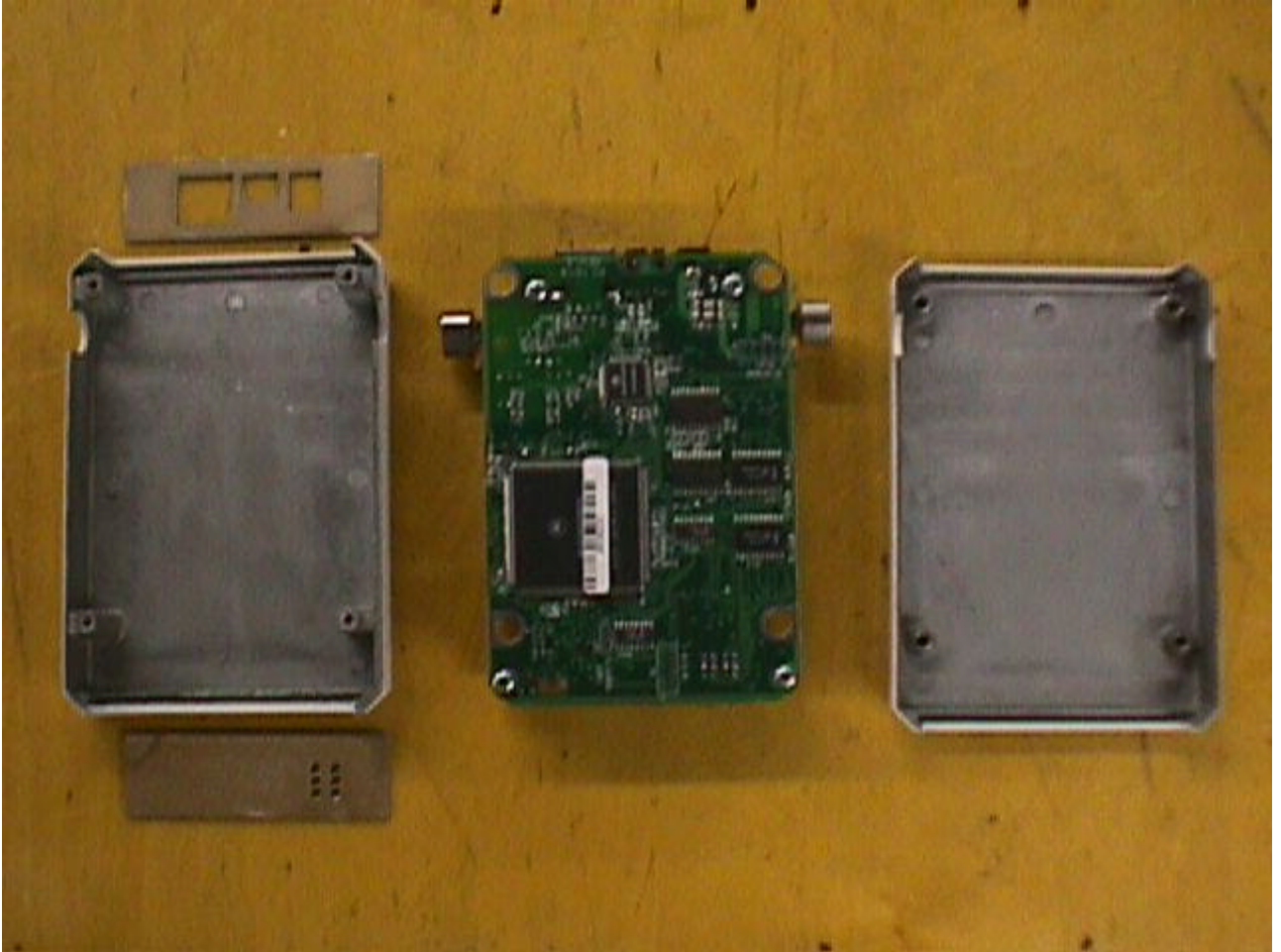
G14: RADIO TRANSCEIVER HOUSING COVER AND RF BOARD SOLDER SIDE WITH SHIELD
