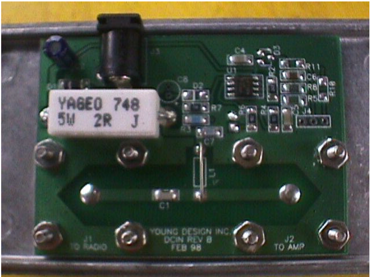
G10: DC POWER INJECTOR COMPONENT SIDE VIEW
