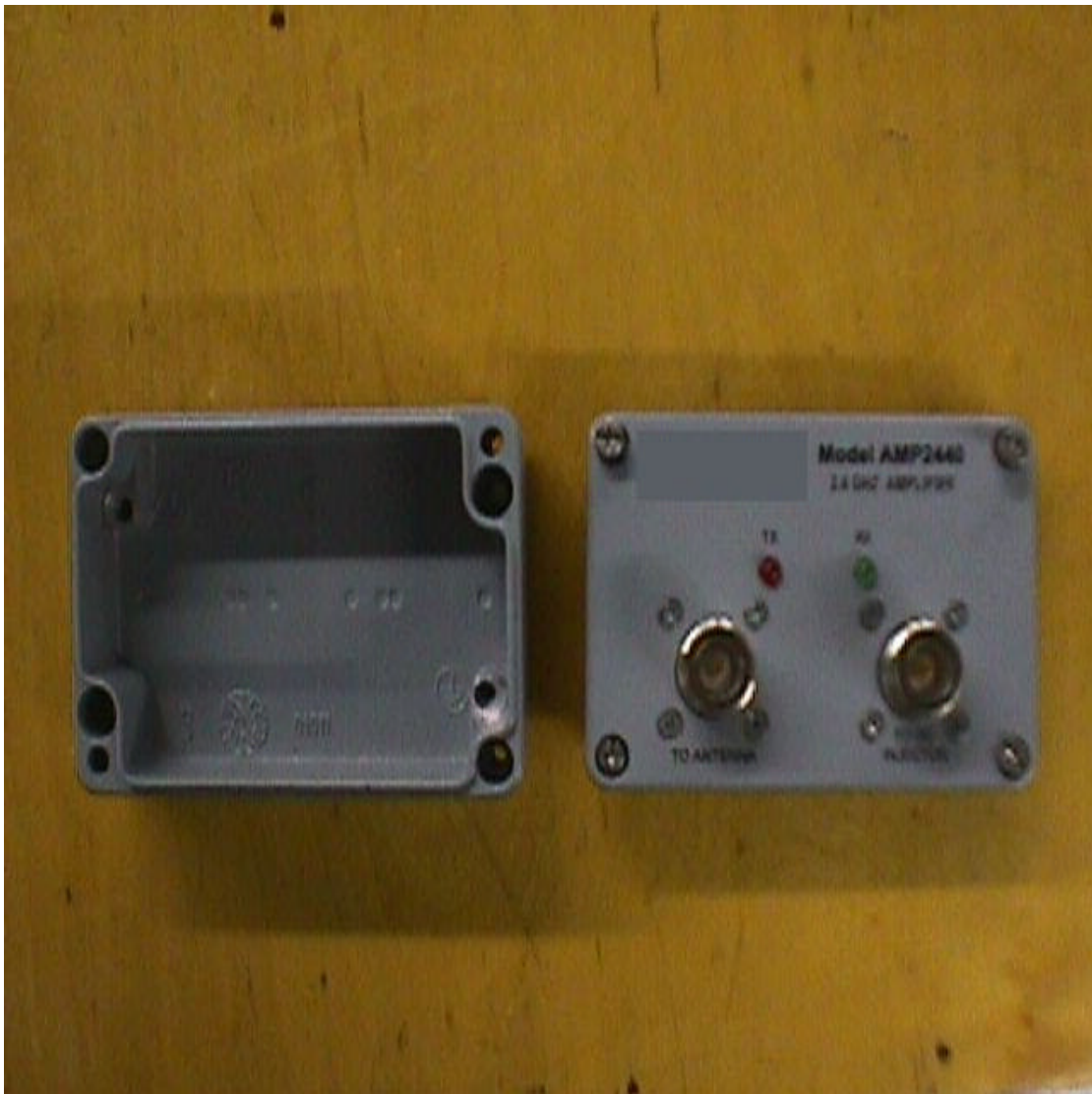
G3: AMPLIFIER TOP VIEW AND INSIDE VIEW OF CHASSIS
