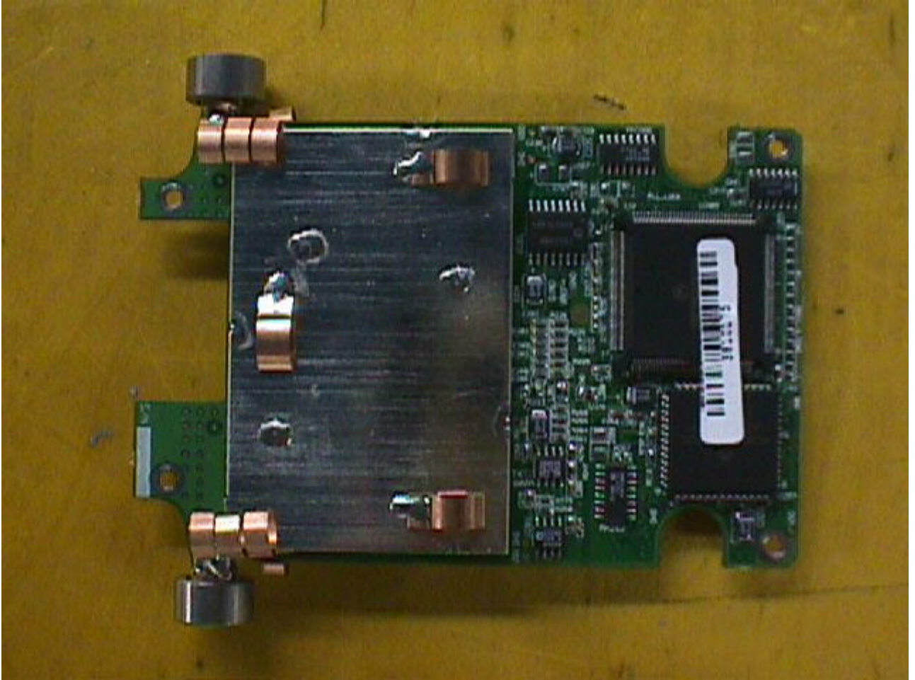
G15: RADIO TRANSCEIVER RF BOARD COMPONENT SIDE WITH SHIELD
