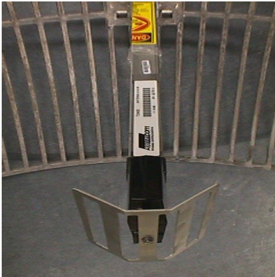
G23: UNI-24 UNI DIRECTIONAL ANTENNA CLOSE UP
