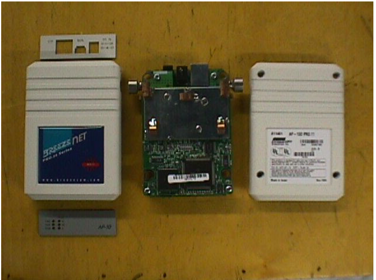
G13: RADIO TRANSCEIVER HOUSING AND RF BOARD COMPONENT SIDE WITH SHIELD
