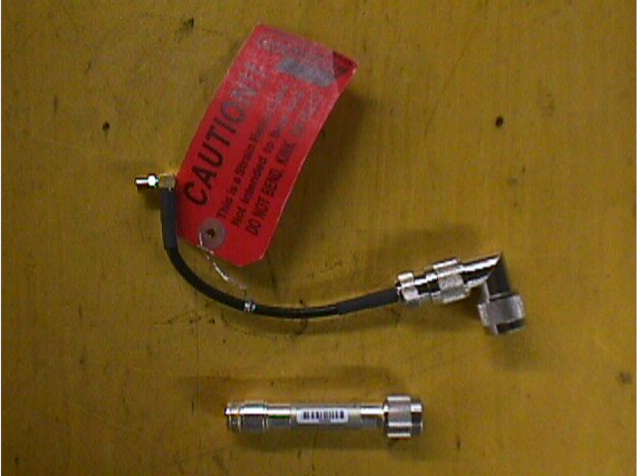
G11: 4" COAX CABLE AND FILTER
