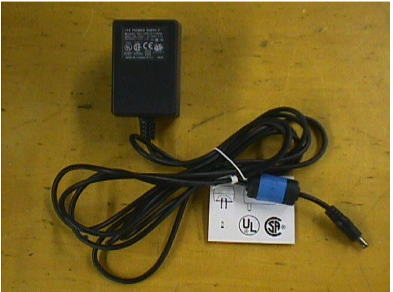
G20: TRANSCEIVER AC/DC POWER SUPPLY
