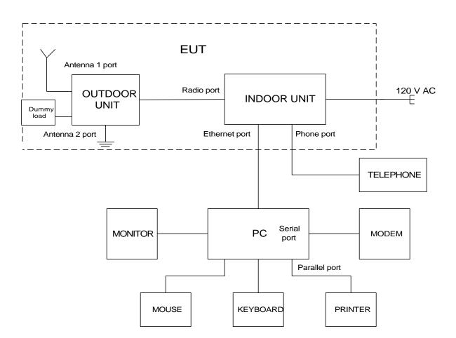
Figure 1.2 AU-O, SU-O-xD and SU-O-xD1V test configuration
