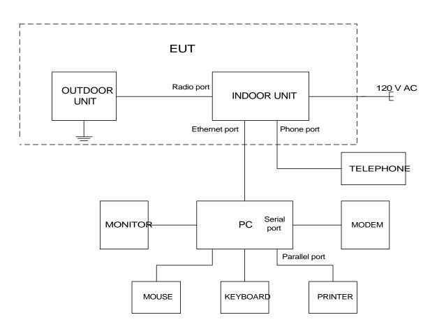
Figure 1.1 SU-A-xD and SU-A-xD1V test configuration
