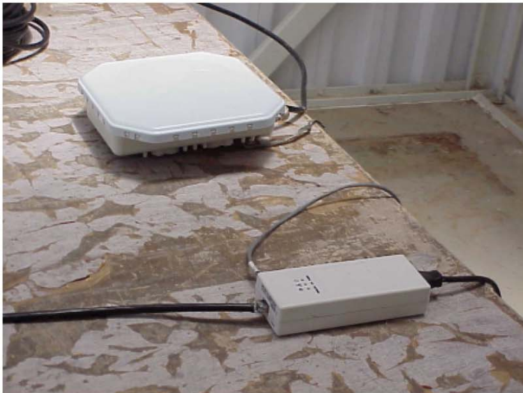
Photo # 5. Subscriber Unit + Power Supply (IDU) Radiated emission test on open site Front / side / overall view
