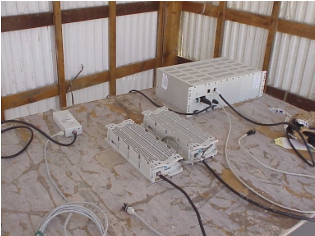
Photo # 6. Base Station + Subscriber Unit Radiated emission test on open site
