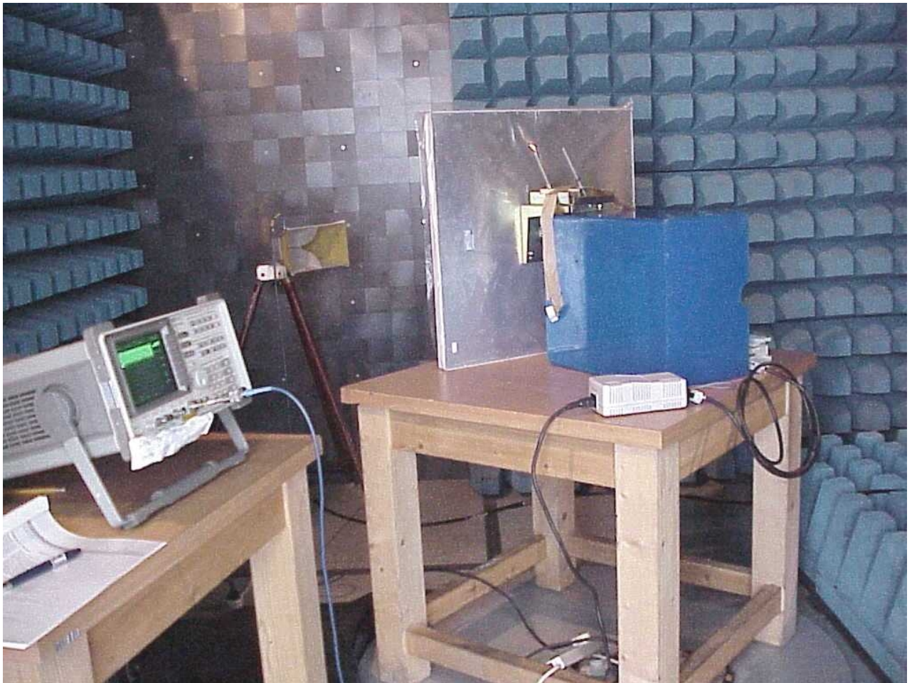
Photo # 1. BreezeNET B unit with Antenna UNI-28-4 P/N 858109. Test setup
