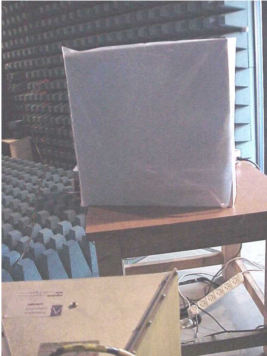
Photo # 2. BreezeNET B unit with Antenna UNI-28-4 P/N 858109. Test setup
