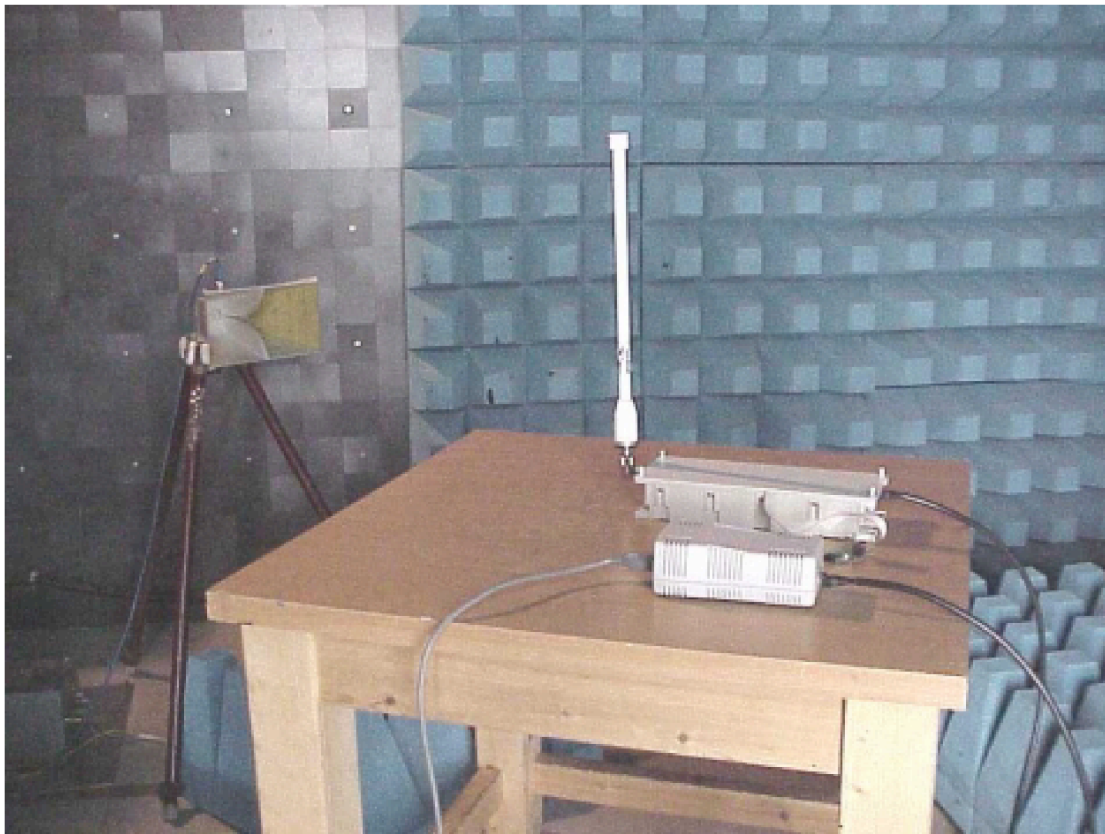
Photo #11 Radio unit with MAXRAD Omni antenna model MFB58008 Spurious emission test
