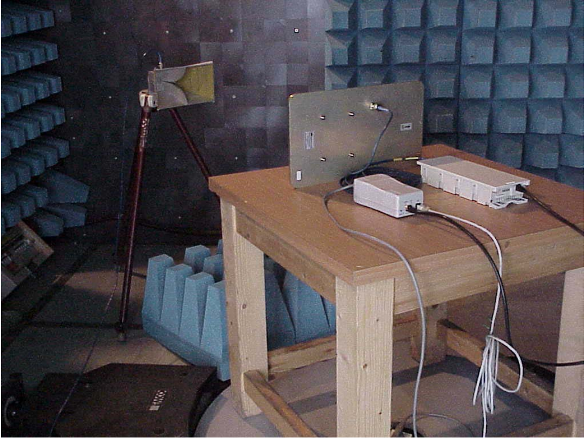
RE 1-26 GHz test set-up detail
