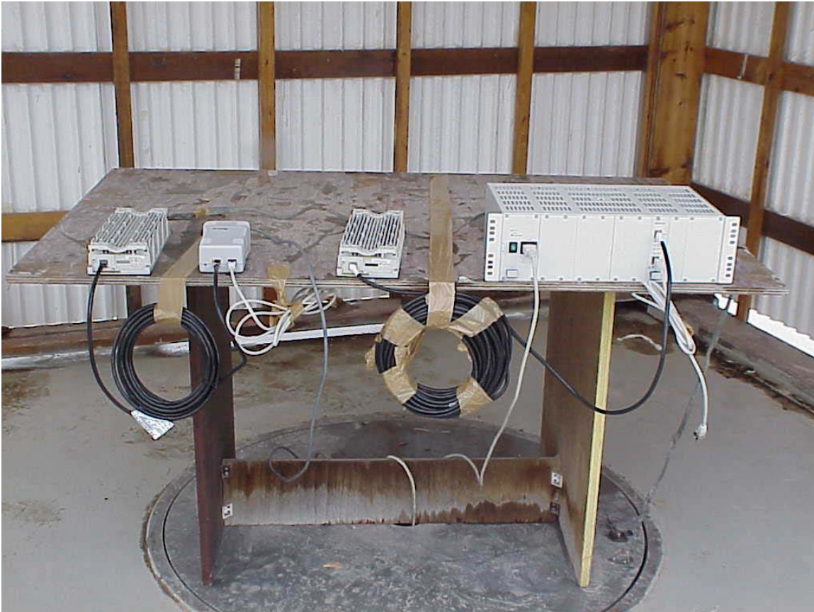
Set-up, system digital radiated emissions test 30 - 1000 MHz
