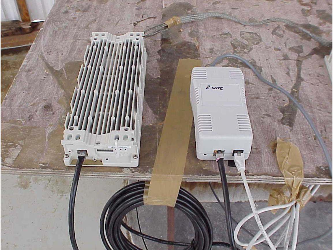
Detail, subscriber IDU and outdoor radio unit connection
