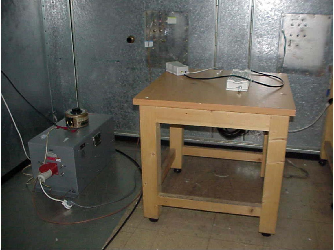
AC line conducted emissions test set-up
