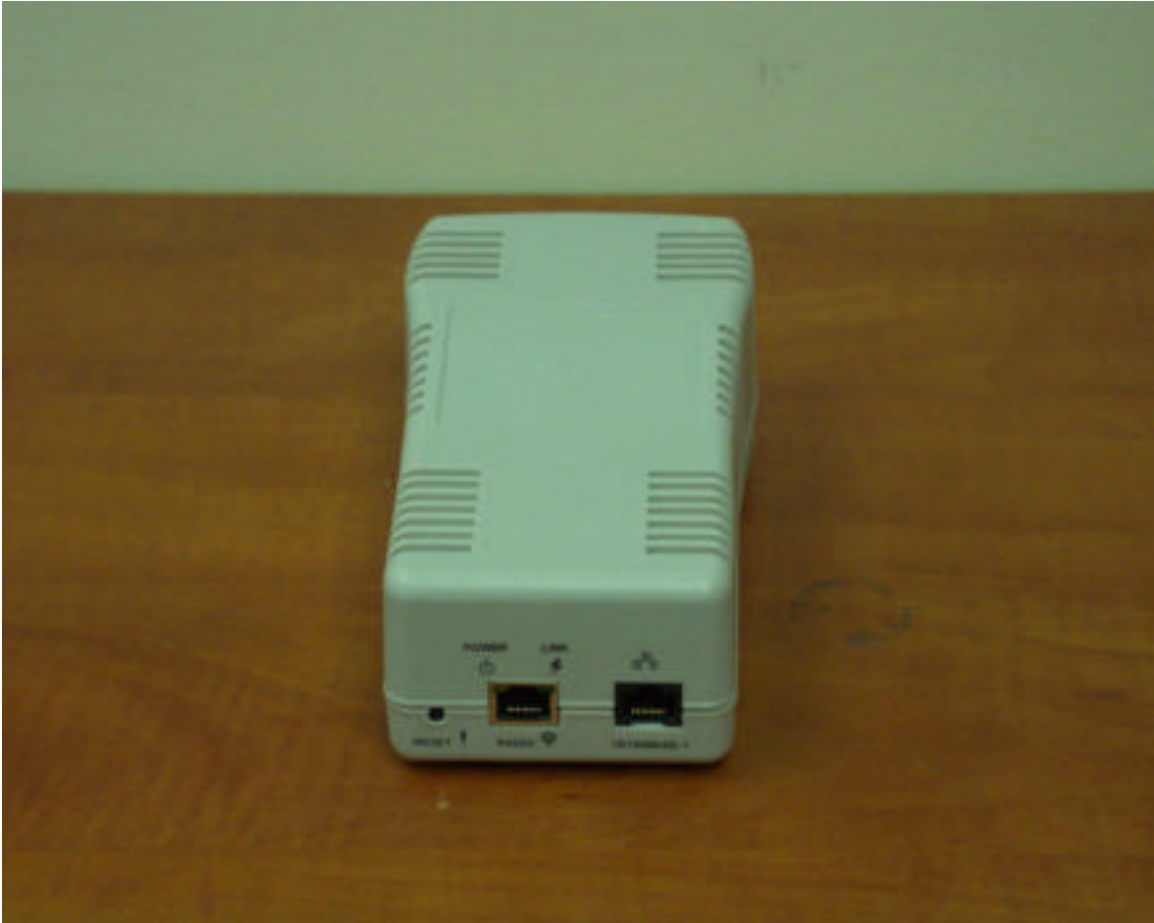
Subscriber IDU, Ethernet and Outdoor Radio Unit Connection Side
