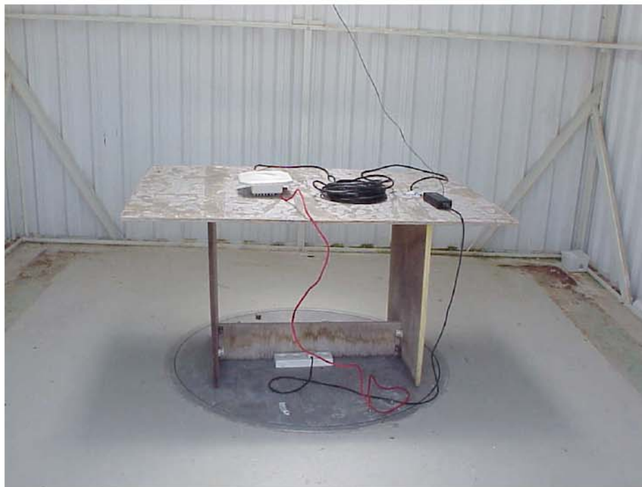
Photo 1. Test setup on OATS. Subscribe unit configuration.
