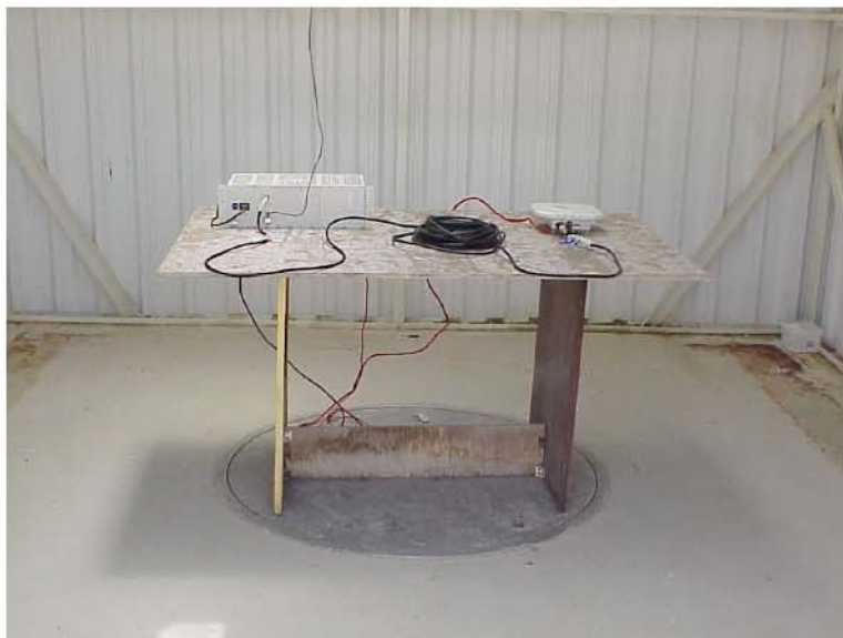
Photo 2. Test setup on OATS. Base station configuration.
