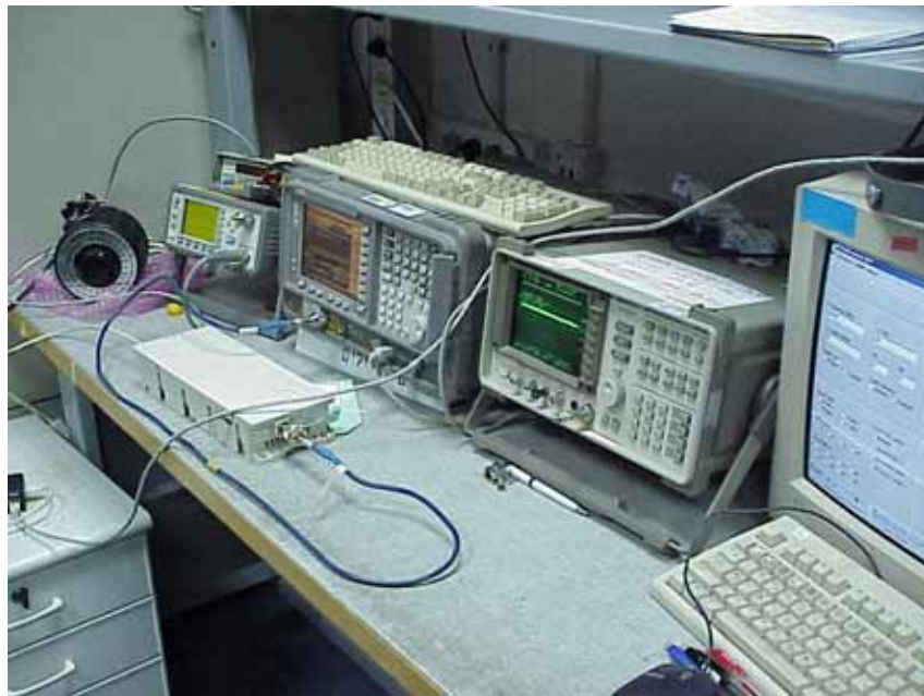
Photo # 5. Conducted measurements setup.
