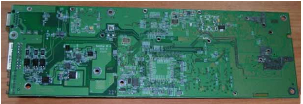
Photo # 3. Radio Unit. PCB print side
