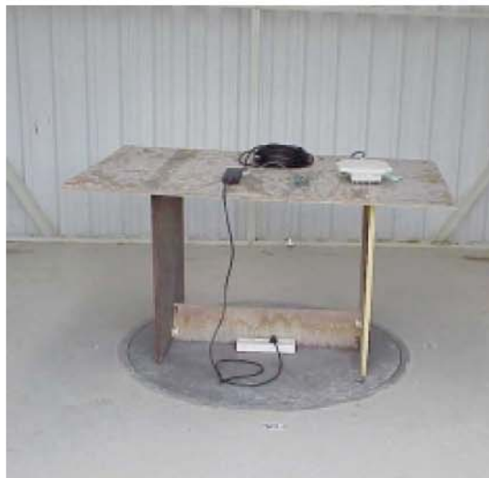
Photo # 7. Subscriber Unit Radiated emission test on open site
