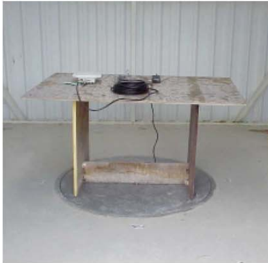
Photo # 6. Subscriber Unit Radiated emission test on open site
