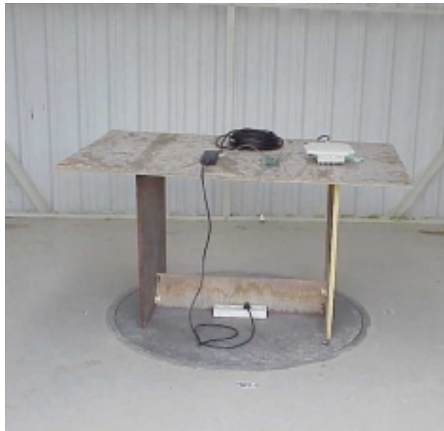
Photo # 7. Subscriber Unit Radiated emission test on open site
