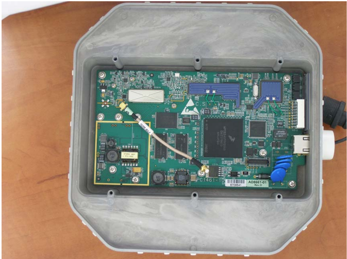
ODU , PCB view after antenna removed
