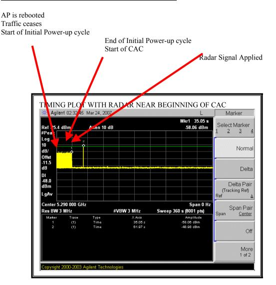
The radar signal is applied (61.97 - 35.05) = 26.69 seconds after reboot, which is (26.69 - 21.3) = 5.39 seconds after the completion of the initial power-up cycle / start of the CAC period.
