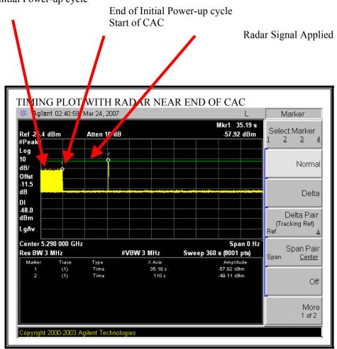
The radar signal is applied (110 - 35.19) = 74.81 seconds after reboot, which is (78.41 - 21.3) = 53.51 seconds after the completion of the initial power-up cycle / start of the CAC period.
