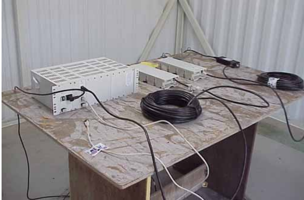
Photo # 8. Base Station + Subscriber Unit Radiated emission test on open site
