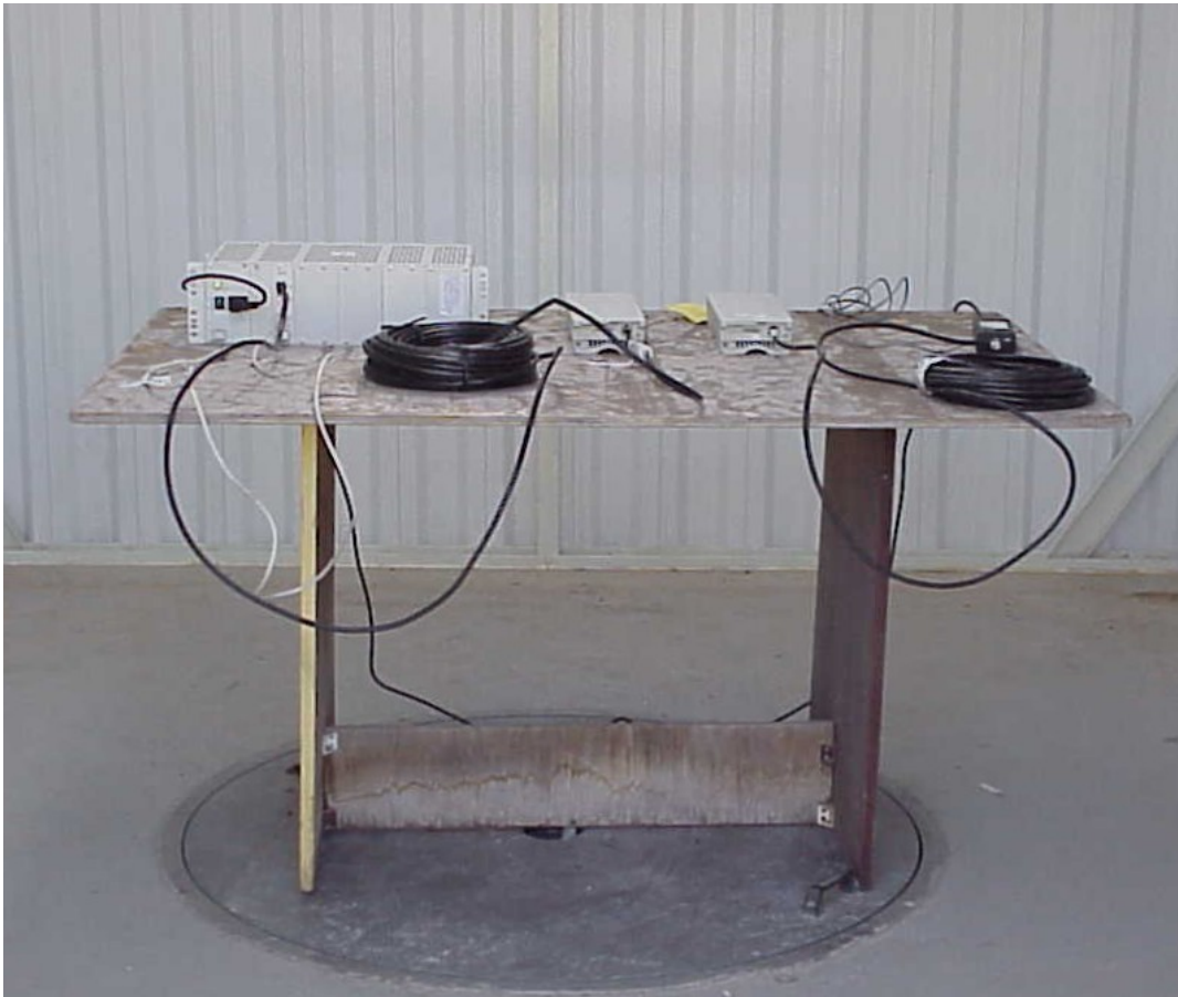
Photo # 6. Base Station + Subscriber Unit Radiated emission test on open site
