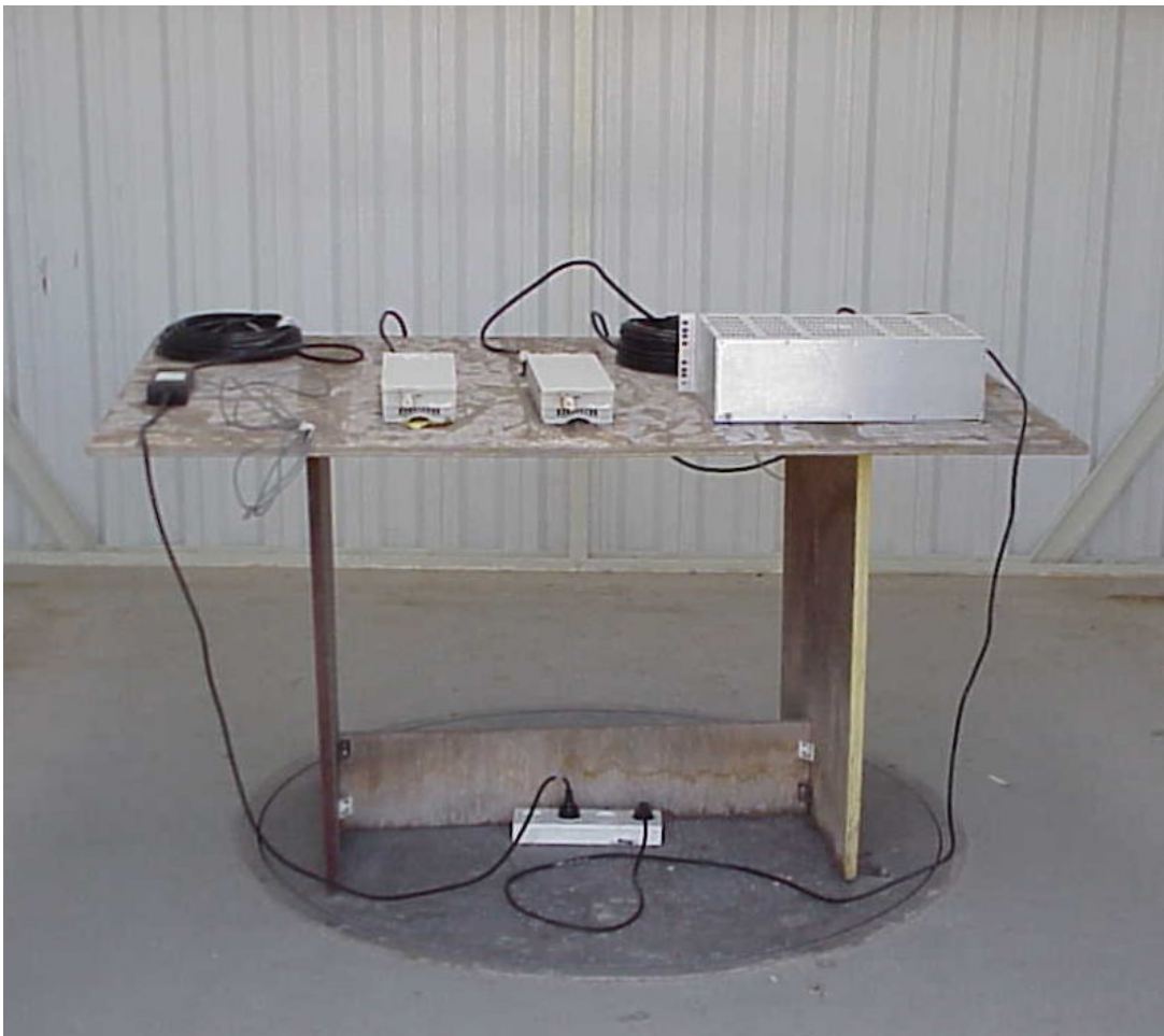
Photo # 7. Base Station + Subscriber Unit Radiated emission test on open site
