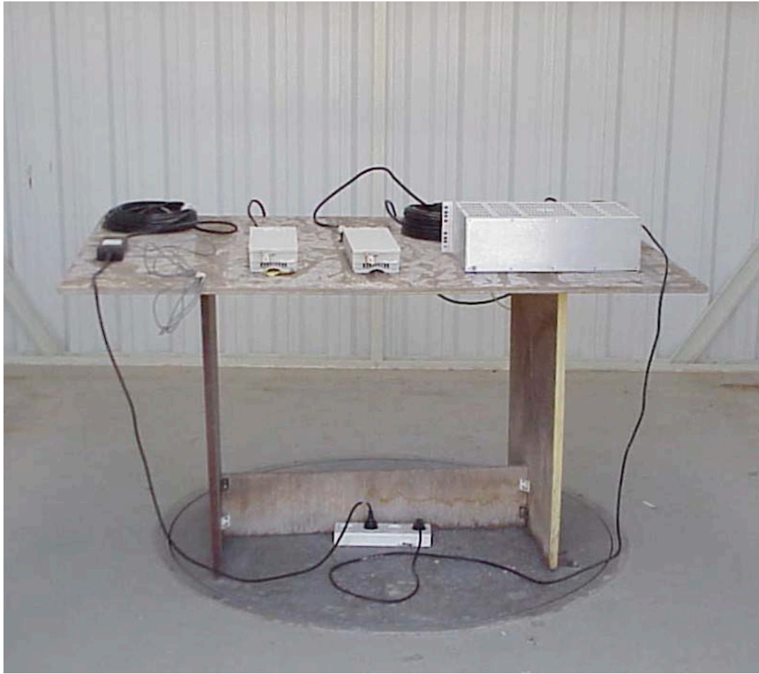
Photo# 3. Radiated emission open site test
